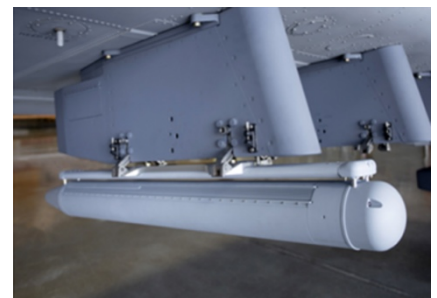
Synthetic Aperture Radar (SAR) 58 inches long, 24 pounds, 275 watts
